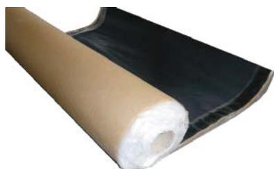
Solsheet Self Adhesive Gas Membrane is designed to prevent the transmission of carbon dioxide, radon and methane gases in tanking applications or where hydrostatic pressure is present. This is in addition to the products usage as a damp proof membrane.
